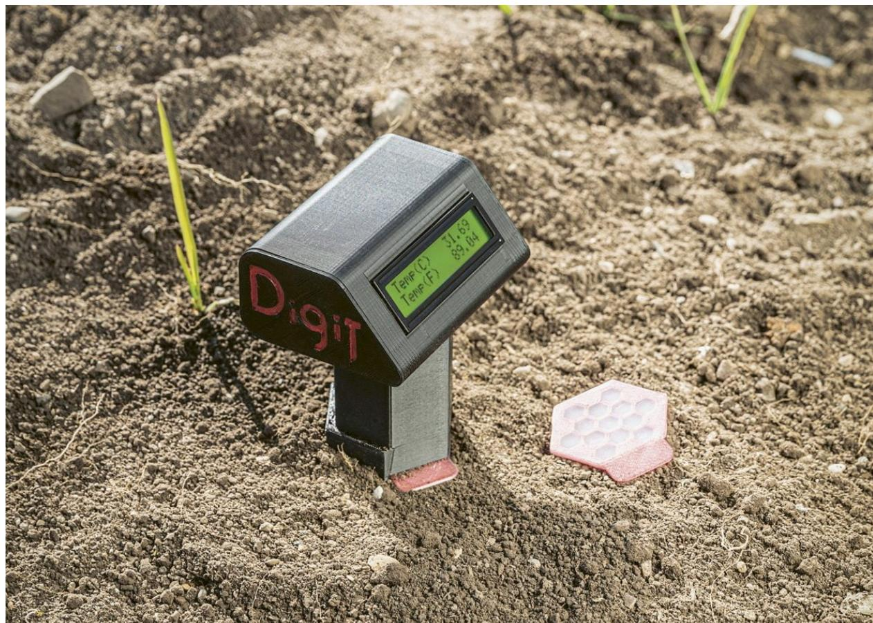
How healthy is my soil? The Digit Soil sensor provides answers by determining the activity of soil enzymes involved in natural carbon, nitrogen, phosphorous and sulphur cycles.
