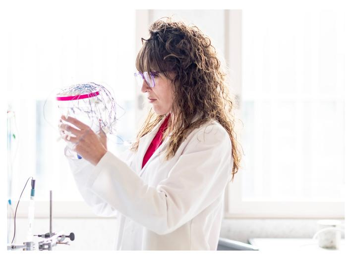
DuraMon's novel pH sensors are immersed in alkaline solution to calibrate before being placed in concrete. © ETH Foundation / Daniel Winkler 31 August 2023
