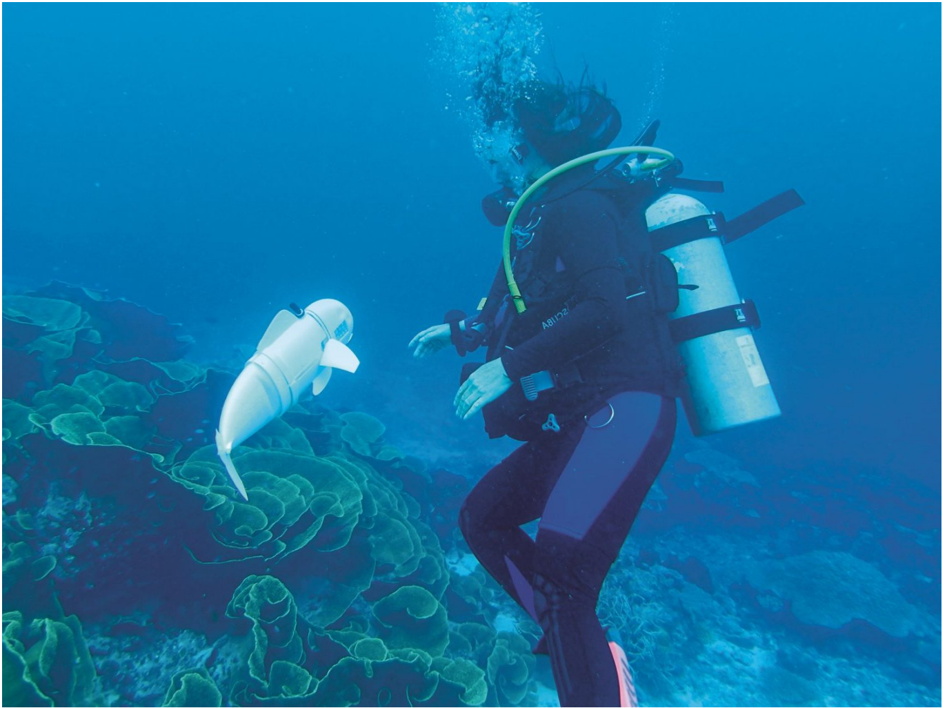
The underwater robot SoFi, which emulates the movement of fish, enables close-up recordings of the marine world to be made. © Joseph Del Preto 27 June 2023
