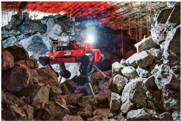
ANYmal's batteries last for two hours of autonomous work in a harsh environment. The robot is equipped with lidar sensors, visual and thermal cameras, microphones and gas-detecting sensors.
