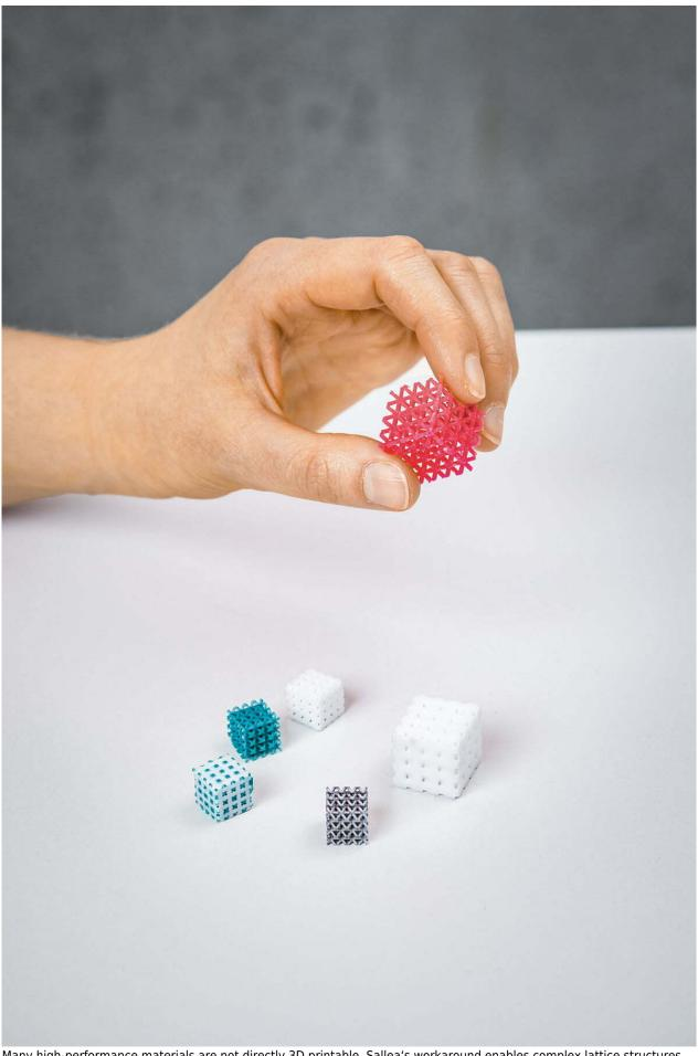
Many high-performance materials are not directly 3D printable. Sallea's workaround enables complex lattice structures to be made from these materials too.
